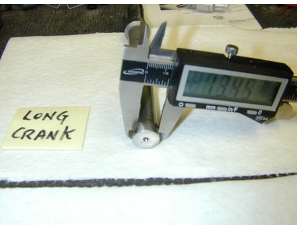
Mike Cecchini: Same measurement on the left end of the crank. 13.45 mm
