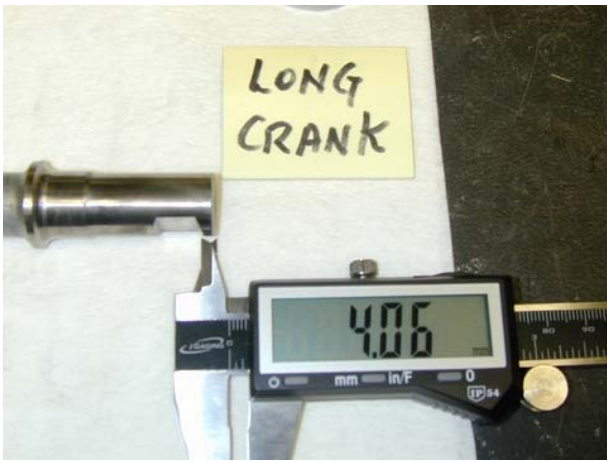
Mike Cecchini: Right end of the crank..... from the end of the crank to the floor of the cut-out.....not the angled part
