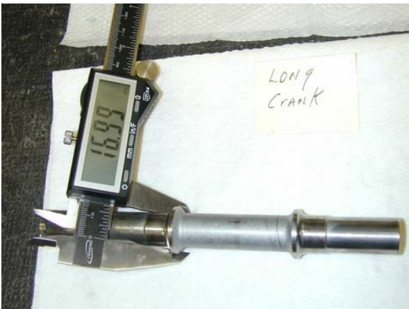
Mike Cecchini: OD of the left end bearing surface
