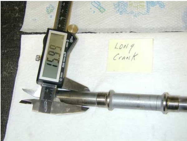
Mike Cecchini: OD of the left end of the crank
