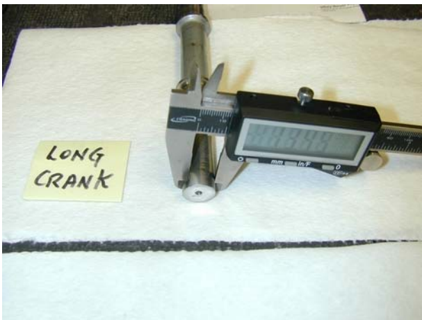
Mike Cecchini: OD of the shaft when measured from the floor of the cut-out. It's hard to read but it's 13.45 mm
