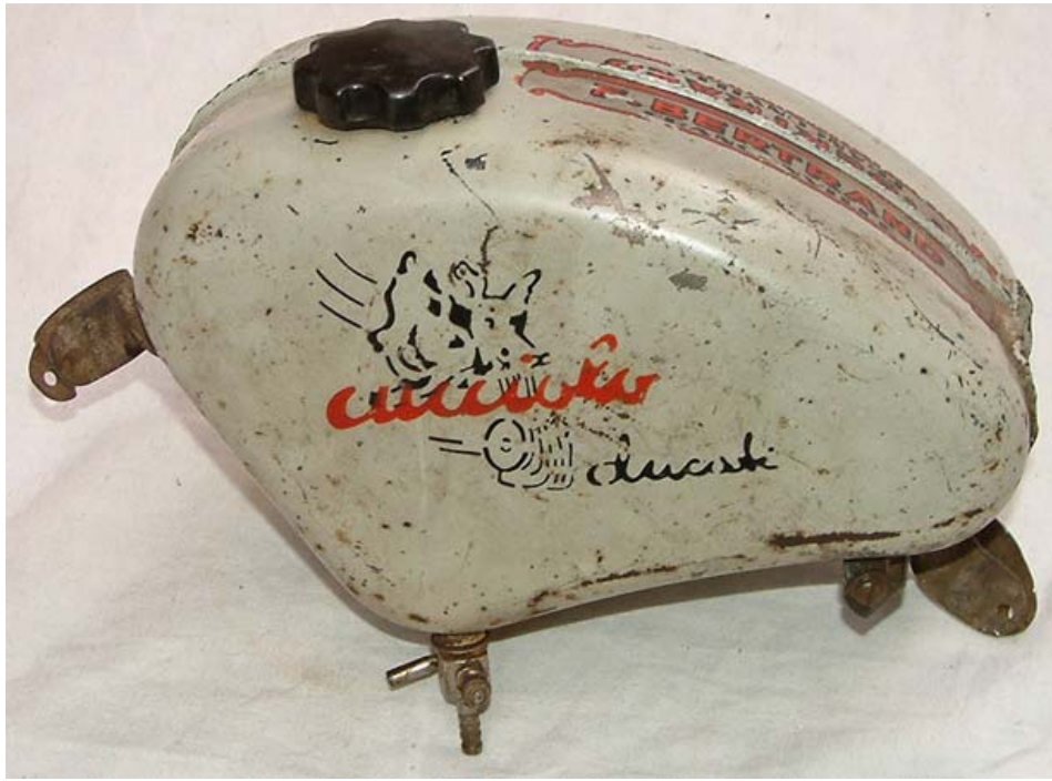
Original Tank with alternative fixing brackets
