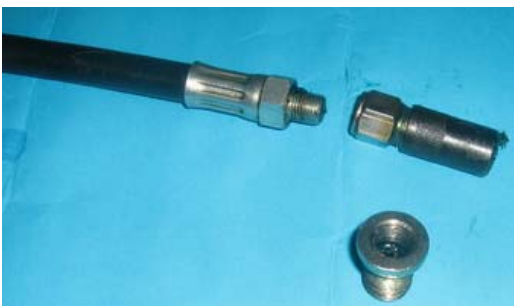
Grease gun with modified spark plug
