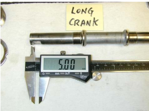
Mike Cecchini: From the end of the crank to the start of the cut-out for the locating/locking pin that holds the bicycle pedal arm to the crank..... not the angled area, but the start of the floor of the cut-out.
