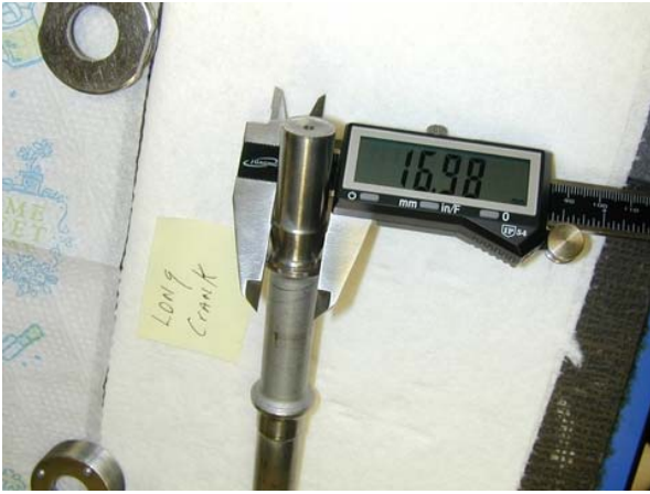
Mike Cecchini: OD of the crank roller surface.
